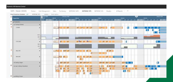
Shows all manufacturing data structured by the registered resources. The production order routing lines are colored by the status; visual alerts appear in case an operation moves past the due date. You can complement the view by showing the amount of hours or units assigned per resource, this is the histogram, or capacity load chart.
